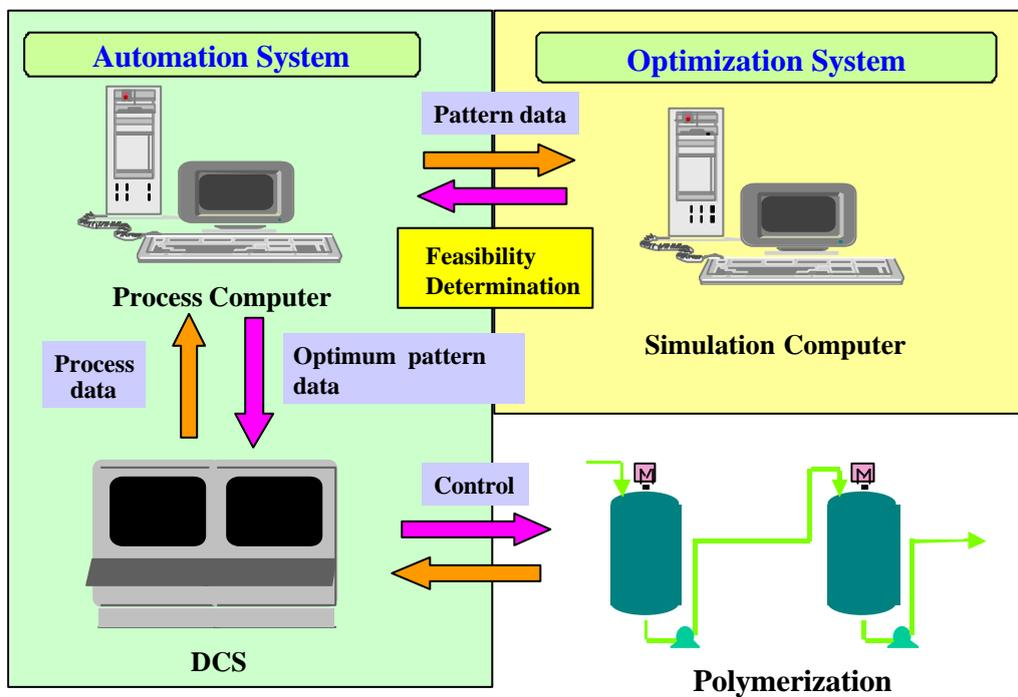
Figure 4. System Structure for Automatic Grade Transitions
