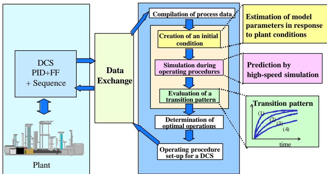
Figure 5. Determination of Optimal Operating Procedures and Integration with Control Systems
