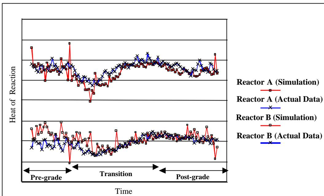
Figure 6. Heat of Reaction during a Grade Transition
