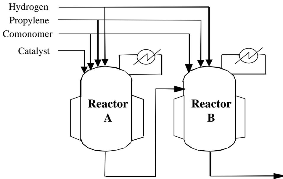
Figure 3. Continuous Liquid-Pool Process Flow
